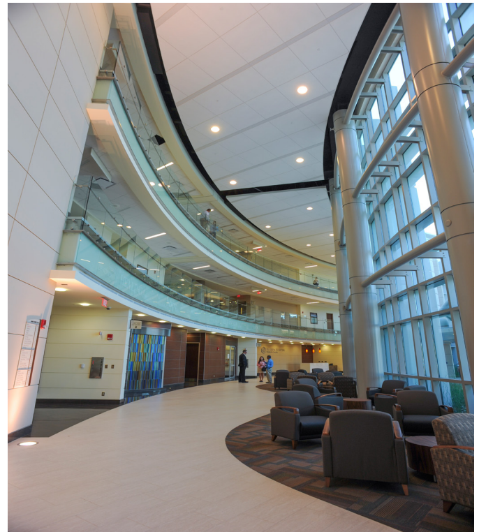
Slightly curved hallways grant nurses the ability to see down the length of the hallway from their stations.
